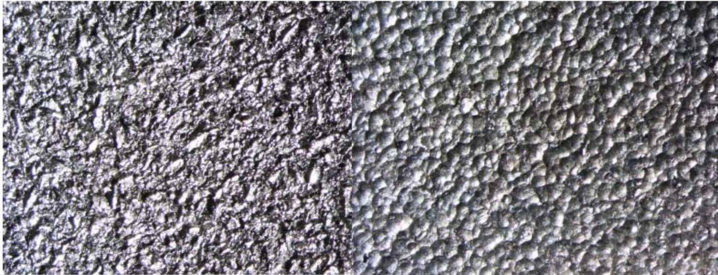
STEEL SUBSTRATE BLASTED WITH GL-25 STEEL GRIT
